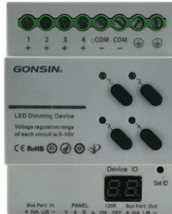
LED dimming control used in various occasions, supporting 0-10V control dimming, with rail design, and can be installed in standard distribution box. RS485 or can communication mode can be selected, and multiple groups of state saving and recovery functions are available. It is suitable for LED dimming under central control management and other application scenarios supporting 0-10V control to realize various intelligent controls.
